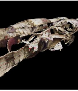
A twin bored, segmentally lined tunnel being constructed in soft marine deposit ground completely collapsed in March 2020 during cross-passage construction. Due to the soft ground conditions, the area at the cross-passage location was pretreated with grout prior to tunnel boring machine (TBM) operations. Subsequently, cross-passage construction commenced using an open-face excavation methodology.
